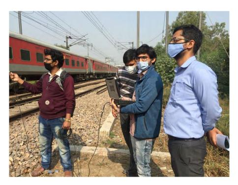
Photo 3.7 Noise Monitoring at Railway Track
