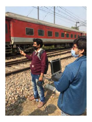
Photo 3.8 Noise Monitoring at Railway Track
