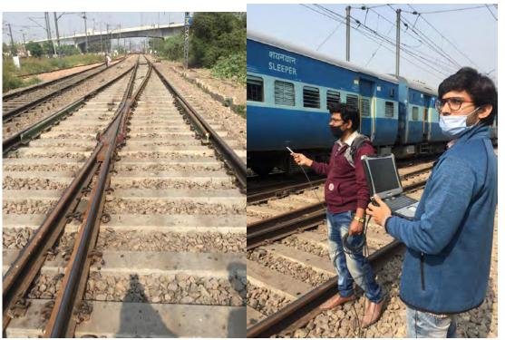
Photo 3.4 Noise Monitoring at Railway Track Railway Track
